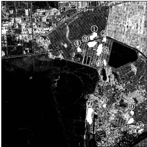
图 6 从交叉熵差异图像中检测出的变化区域 Fig. 6 The change detection results from the differential image of cross-entropy
