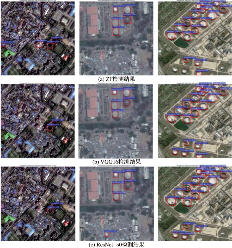
图 7 不同模型油罐识别效果比较 Fig.7 The oil tank detection results of the three models
