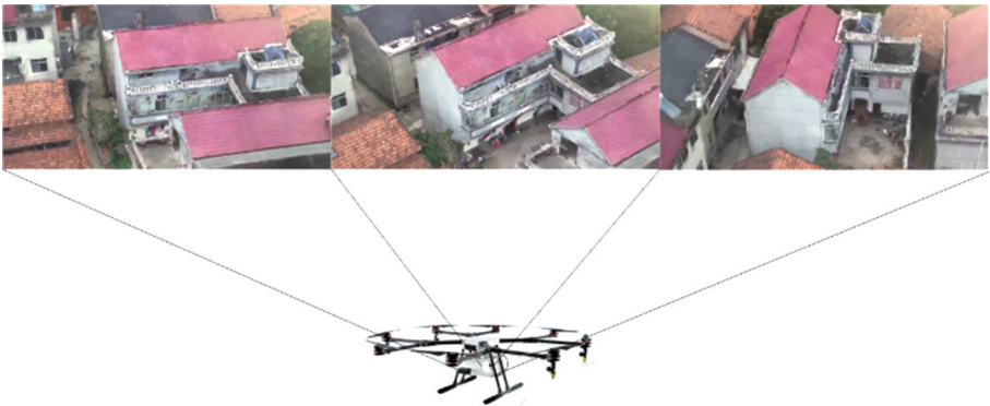
图 7 基于无人机倾斜摄影测量的三维立体建模 Fig.7 UAV-based oblique photogrammetry for 3-D building modelling
